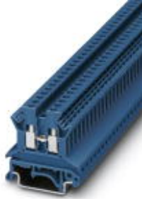
Feed-through terminal block, Connection method: Screw connection, Cross section: 0.2 mm 2 - 4 mm 2 , AWG: 24 - 12, Width: 5.2 mm, Color: blue, Mounting type: NS 35/7,5, NS 35/15
