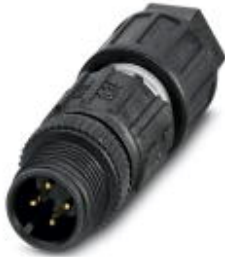
Sensor/actuator connector, 4-position, Plug straight M12, A-coded, Insulation displacement connection, Knurl material: Plastic, External cable diameter 3.5 mm ... 6 mm
