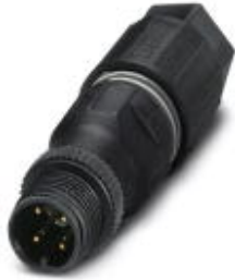
Sensor/actuator connector, 4-position, Plug straight M12, A-coded, Insulation displacement connection, Knurl material: Plastic, External cable diameter 4 mm ... 8 mm
