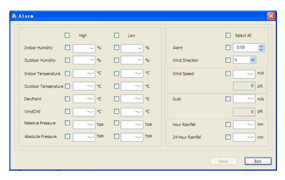
This section is used to set the desired time, high or low alarm value for the base unit, as well as able or disable the corresponding alarm function. Once you made your choice, choose Save to make the setting effective. If you don't want to make any change, just press Cancel and exit without change.
