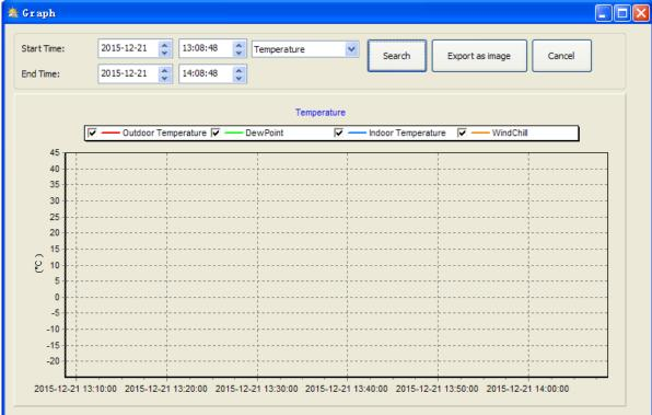
With the Export as image button, you can export the selected graph into .jpeg format file. You can change the Y axel by scrolling the mouse up and down roller.
