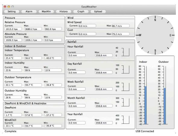
The functions of MAC OS are the same to the windows version. Once the device is connected to MAC PC by USB cable, settings, alarms of all weather parameter can be done here. Max/Min record, all history record can be viewed. History records can be exported as excel or PDF file as well.
