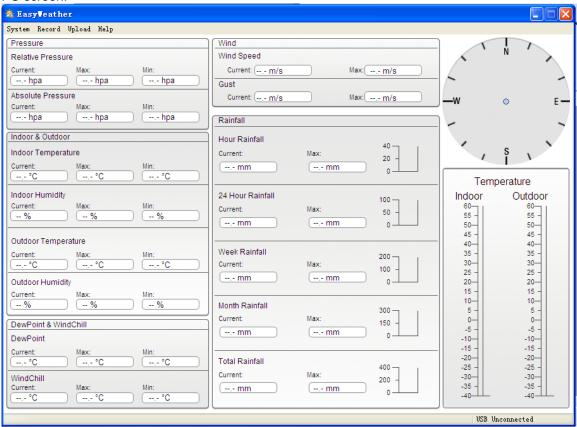
All the settings from the base unit is mirrored into the PC software, so once you have done your setting on the base unit, then you don't need to make any setting changes on the PC software. However you can still easily make any setting changes you wanted from the PC and download the changes into the base station(the setting change will be refreshed when next full minute arrives on the base station).
