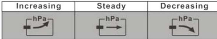
**Note :** It is only possible to measure the barometric pressure trend properly when the unit remains at the same altitude location. When moving around at different altitudes within a short period of time, the air pressure and the barometric pressure will change. The pressure trend will only be correct and regular if the unit remains at a constant location altitude for 24 hours or more.
