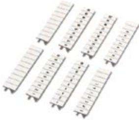
Zack marker strip, Strip, white, labeled, Printed horizontally: Consecutive numbers, Mounting type: Snap into tall marker groove, For terminal block width: 5.2 mm, Lettering field: 10.5 x 5.15 mm
