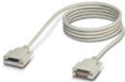
Assembled D-SUB cable shielded, 15-pos., stranded (7-wire), cable color RAL 7000 (gray), IP20 degree of protection, head 1 with socket shell 2 and straight cable outlet, head 2 with pin shell 2 and straight cable outlet, length: 2 m
