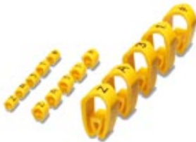
Conductor marking collar, yellow, Unlabeled, Mounting type: Thread on, Cable diameter: 1.9-3.8 mm
