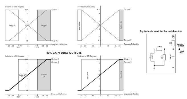
The two switch outputs are configured as 'Open Drain' with a 1K5 pull-up to the 5V.
