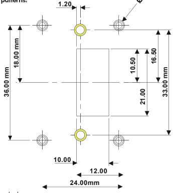
The Paddle is fitted with M3 bushes in all six positions, as standard.
