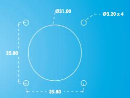
The joystick flange is mounted beneath the panel and the base of the gaiter must be brought through the panel cut-out and held in place with the circular bezel.
