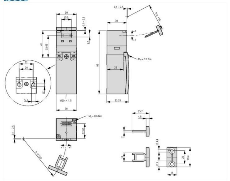
Switch must not be used as a mechanical stop
