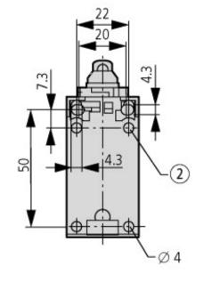
(1) Tightening torque of cover screws: 0.8 Nm ±0.2 Nm (2) only with LS (insulated version) (3) Fixing screws 2 x M4 ≧ 30 M<sub>A</sub> = 1.5 Nm
