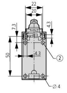
$\begin{array}{l} ( \mbox{$1$} Tightening torque of cover screws: 0.8 Nm \pm 0.2 Nm $$$$ 0.8 Nm \pm 0.2 Nm $$$$$ only with LS (insulated version) $$ only with LS (insulated version) $$ Fixing screws 2 x M4 $$ 30 $$ MA = 1.5 Nm $$ \end{tabular}$
