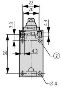
$\begin{array}{l} \textcircled{1}{1} \mbox{ Tightening torque of cover screws: 0.8 Nm \pm 0.2 Nm } \\ \hline \textcircled{0}{0} \mbox{ only with LS (insulated version)} \\ \hline \textcircled{1}{3} \mbox{ Fixing screws 2 x M4 } \geqq \mbox{ 30 } \\ \hline M_A = 1.5 \mbox{ Nm} \end{array}$
