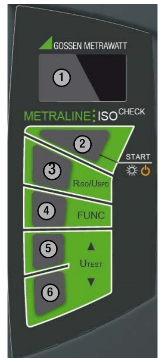
Figure 2.3: Control Panel and OLED Display
