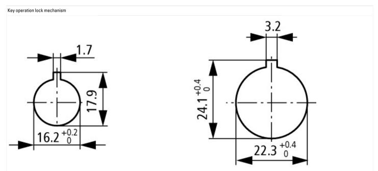
Door drilling dimensions Drilling dimensions: either 16.2 mm = without reduction  $\triangleq$  RMQ16 or 22.3 mm = with reduction  $\triangleq$  RMQ Titan
