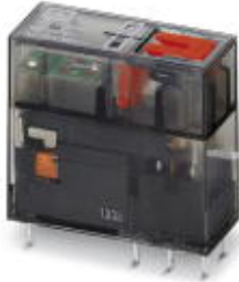
Plug-in miniature relay, with power contact, 1 PDT, test button, mechanical switch position indicator, status LED, input voltage 230 V AC
