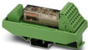
Universal safety relay with forcibly guided contacts, spring-cage connection, 4 N/O contacts, 2 N/C contacts, width: 40 mm
