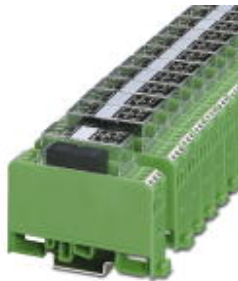
Relay module, with soldered-in miniature switching relay, contact (AgNi): Medium to large loads, double A2 connection, 1 PDT, 230 V AC/DC input voltage
