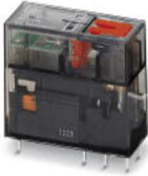
Plug-in miniature relay, with power contact, 2 PDTs, test button, mechanical switch position indicator, status LED, coil voltage 230 V AC
