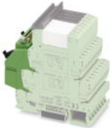
V8L-INPUT adapter for eight 6.2 mm PLC interfaces (1 PDT, etc./see "Supplementary Products"). 14-pos. flat-ribbon cable connection for the PLC system cabling, control logic: Minus switching
