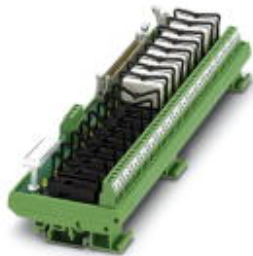
VARIOFACE output module, with 16 miniature relays, 1 PDT each, plugged, for 24 V DC (basic module, including relays)
