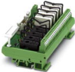
VARIOFACE output module, with 8 miniature relays, 1 PDT each, plugged, for 24 V DC (including relays)
