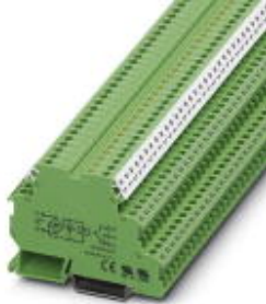
Relay terminal block, with soldered-in miniature relays, contact (AgNi+Au): small to medium loads, 1 N/O contact, input voltage 24 V AC/DC, for assembly on NS 35/7.5, terminal width 6.2 mm
