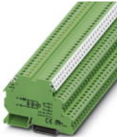
Relay terminal block, with soldered-in miniature power relay, contacts (AgSnO): medium to large loads, 1 PDT, input voltage 24 V DC, for assembly on NS 35/7.5, terminal width 6.2 mm
