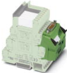
V8-OUTPUT adapter for eight 6.2 mm PLC interfaces (1 PDT, etc./see "Additional Products"). 15-pin D-SUB male connector, control logic: Positive switching
