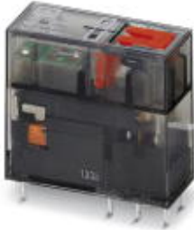
Plug-in miniature relay, with power contact, 1 PDT, test button, mechanical switch position indicator, status LED, input voltage 120 V AC
