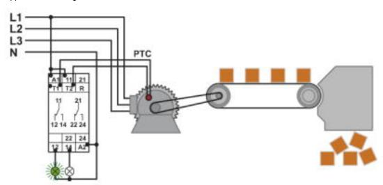
Monitoring of motor winding temperatures
