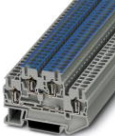
Feed-through terminal block, Cross section: 0.08 mm 2 - 4 mm 2 , AWG: 28 - 12, Connection type: Spring-cage connection, Width: 5.2 mm, Color: gray, Mounting type: NS 35/7,5, NS 35/15
