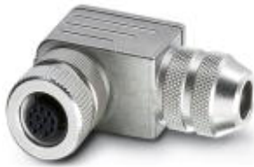
Connector, Universal, 12-position, shielded, Socket angled M12, A-coded, Solder connection, Knurl material: Zinc die-cast, nickel-plated, Cable gland Pg9, External cable diameter 6 mm ... 8 mm
