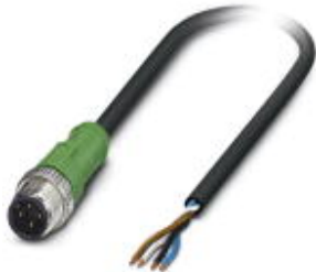
Sensor/Actuator cable, 4-position, PVC, Black RAL 9005, Plug straight M12, A - standard, on Free cable end, Cable length: 2 m
