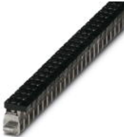
Connection terminal block, Connection method Screw connection, Load current : 76 A, Cross section: 1.5 mm 2 - 16 mm 2 , Width: 9.8 mm, Color: black
