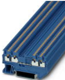
Feed-through terminal block, Connection method: Push-in connection, Cross section: 0.14 mm 2 - 1.5 mm 2 , AWG: 26 - 16, Width: 3.5 mm, Color: blue, Mounting type: NS 35/7,5, NS 35/15
