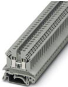
Feed-through terminal block, Connection method: Screw connection, Cross section: 0.2 mm 2 - 4 mm 2 , AWG: 24 - 12, Width: 6.2 mm, Color: gray, Mounting type: NS 35/7,5, NS 35/15
