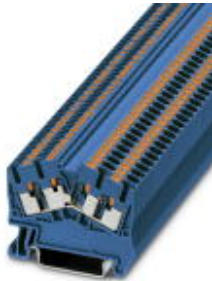
Feed-through terminal block, Connection method: Push-in connection, Cross section: 0.14 mm 2 - 4 mm 2 , AWG: 26 - 12, Width: 5.2 mm, Color: blue, Mounting type: NS 35/7,5, NS 35/15
