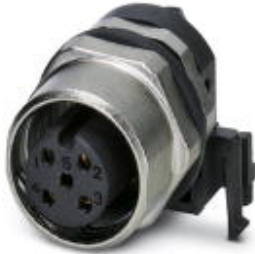
Sensor/actuator flush-type connector, socket, 4-pos., M12 SPEEDCON, A-coded, rear/screw mounting with M12 thread, with polarity protection, with angled solder connection
