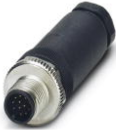
Connector, Universal, 12-position, Plug straight M12, A-coded, Solder connection, Knurl material: Zinc die-cast, nickel-plated, Cable gland Pg9, External cable diameter 6 mm ... 8 mm
