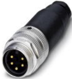
Sensor/actuator connector, male, straight, 5-pos., 7/8", screw connection, metal knurl, cable screw connection Pg9
