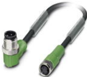
Sensor/Actuator cable, 3-position, PUR halogen-free, Black-gray RAL 7021, Plug angled M12, A-coded, on Socket straight M8, Cable length: 3 m
