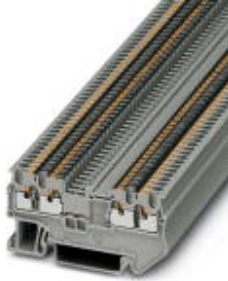
Feed-through terminal block, Connection method: Push-in connection, Cross section: 0.14 mm 2 - 1.5 mm 2 , AWG: 26 - 16, Width: 3.5 mm, Color: gray, Mounting type: NS 35/7,5, NS 35/15
