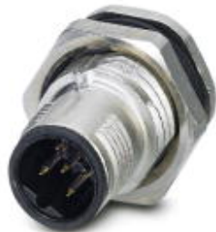
Sensor/actuator flush-type plug, 5-pos., M12-SPEEDCON, shielded, B-coded, rear/screw mounting with Pg9 thread, with straight solder connection
