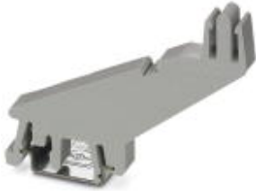
Cover profile holder, 10 mm wide, for mounting on NS 32 or NS 35/7.5, for fixing the holding profile APK-HP, labeling with Zack strip ZB 10
