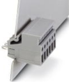
Panel feed-through terminal block, Connection method: Screw connection, Solder/Slip-on connection, Cross section: 0.2 mm 2 - 4 mm 2 , Width: 6.2 mm, Color: gray
