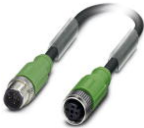
Sensor/Actuator cable, 4-position, PUR halogen-free, Black-gray RAL 7021, shielded, Plug straight M12, A-coded, on Socket straight M12, A-coded, Cable length: 1.5 m
