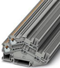
Multi-level terminal block, Cross section: 0.14 mm 2 - 1.5 mm 2 , AWG: 26 - 14, Connection type: Push-in connection, Width: 3.5 mm, Color: gray, Mounting type: NS 35/7,5, NS 35/15
