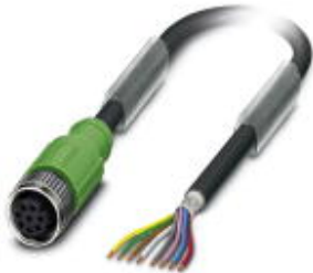
Sensor/Actuator cable, 8-position, PUR halogen-free, Black-gray RAL 7021, shielded, Free cable end, on Socket straight M12, A-coded, Cable length: 1.5 m
