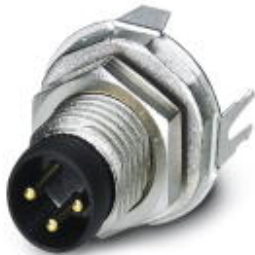
Sensor/actuator flush-type connector, connector, 3-pos. M8, rear/screw mounting with M8 fastening thread, with straight solder connection
