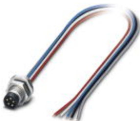
Bus system flush-type connector, plug, DeviceNet, 5-pos., M8, front/screw mounting with M10 fastening thread, with 0.5 m TPE litz wire, 5 x 0.25 mm²
