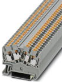
Feed-through terminal block, Connection method: Push-in connection, Cross section: 0.14 mm 2 - 4 mm 2 , AWG: 26 - 12, Width: 5.2 mm, Color: gray, Mounting type: NS 35/7,5, NS 35/15
