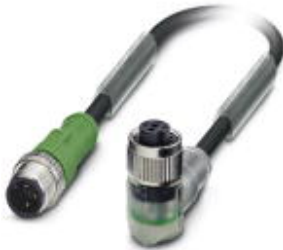
Sensor/Actuator cable, 3-position, PUR, orange RAL 2003, Plug straight M12, A-coded, on Socket angled M12, A-coded, with 2 LEDs, Cable length: 5 m
